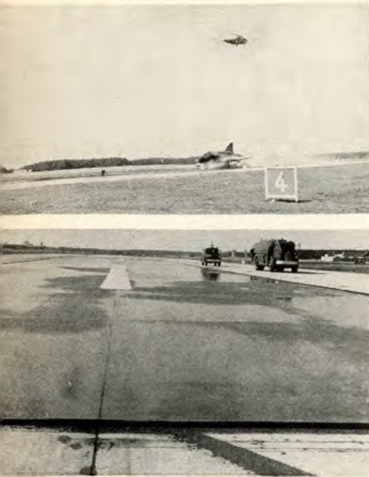
Top photo at left: Maj Clark Price, 68 TFS, George AFB, landing an F-4D on NASA's flooded Wallops Island test runway. The March 1968 tests proved that the transverse runway grooves give a wet runway the same stopping potential as a dry surface. Left, NASA's grooved test runway for the F-4 wet runway tests. Results of this test were overwhelmingly favorable.
